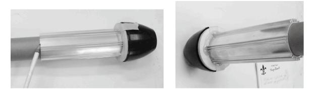
Slide the Groove-Lok onto the motortube and ROTATE it as you bring it down toward the centering ring. This spreads the epoxy evenly. Wipe off excess adhesive and try not to let it pool into the fin channels of the Groove-Lok. Butt it against the aft centering ring. Stand the assembly up right (tailcone down) and allow to cure. See figure above right.
