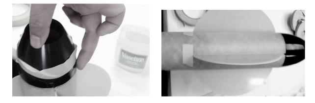
Slide the airframe back onto the fin canister (rotate to align your reference mark). If the slots are slightly longer than your fins, cover the open slots with a small bit of masking tape at the forward end (see Figure above right).
