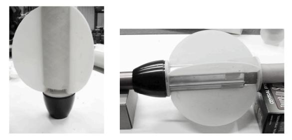
As the epoxy cures, occasionally press the fins into the channels to be sure they are fully seated.
