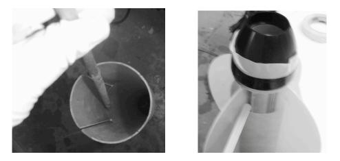
Keeping the airframe in this orientation (slots upward), slide on the fin canister assembly - - but not all the way. Leave about a 1" gap between the airframe and the tailcone (see Figure above right). Using a stick, drip epoxy down the joint where the fin meets the inside of the airframe. Drip additional epoxy on the inside lip of the airframe where it contacts the tailcone and rear centering ring. Use plenty of epoxy for this step.
