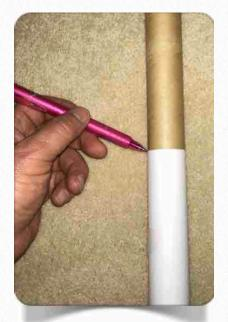
4. Place the Middle Centering Ring onto the motor tube. Measure from the Aft end of the motor tube (the end with the GLR Slimline Retainer attached) 9" and place a mark. Using a piece of paper wrapped around the motor tube, centered on the mark that you made at
