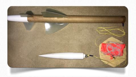
The sequence is a follows: slotted airframe containing the GLR Hardpoint, GLR Kevlar® Shock Cord, GLR Kevlar® Parachute Heat Shield, GLR Kevlar® Shock Cord, swivel, GLR Kevlar® Shock Cord, GLR Pinnacle Nosecone.
