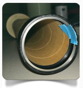
installing it in order to spread the J.B. Weld. Be sure that you only apply the J.B. Weld to the motor tube and NOT to the inside of the GLR Slim-
