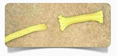
all the way down to the Motor Tube. With one hand hold on to the GLR Kevlar® Shock Cord and with the other hand slide the GLR Kevlar® Sock until is at its half way-point lying on the edge of the airframe, secure it with making tape and/or GLR Aeropoxy.
