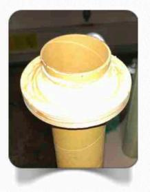
7. It is now very important to place a thick fillet on the Forward and Aft ends of both of the Centering Rings to secure the Centering Rings to the Airframe. Fillets can be created using a variety of materials, Giant Leap Rocketry, LLC
