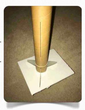
edge of the fin. Insert the fin into the slot until the fin makes contact with the motor tube and transfers the GLR Aeropoxy to the motor tube. You will want to repeat the process 3-5 times to insure that you have good amount of GLR Aeropoxy contacting the fin / motor tube interface. In addition you can drip some GLR Aeropoxy through the slot. Once you have your fins in place, slide the cardboard fin guid down the airframe onto the fins to insure their correct position. Allow to completely set.
