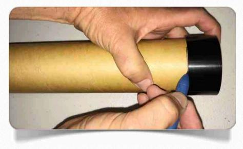
3. Mix some J.B.Weld (and only J.B Weld - do not use epoxy!) and apply it to the aft end of the motor tube, to the pencil mark of the motor tube. Then, install the GLR Slimline Motor Re-
