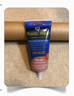
trude a small amount of the DAP Plastic Wood and trace the fine grooves of the Phenolic Airframe and deposit the DAP Plastic Wood into the groves. Be consrervitive because all that is not in the grove must be sanded away. That said, the material does shrink a bit as it drys, so it must be left a little high. When the DAP Plastic Wood is completely set up,
