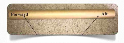
1. Test fit the GLR Slimline Motor Retainer on the Aft end of the 29mm motor tube. Be sure that the GLR Slimline Motor Retainer goes onto the motor tube and seats completely. If the GLR Slimline Motor Retainer is seated completely, you will not have any of the epoxy bonding rings of the GLR Slimline Motor Retainer exposed and the motor tube will rest on the the built-in shoulder stop of the GLR Slim-
