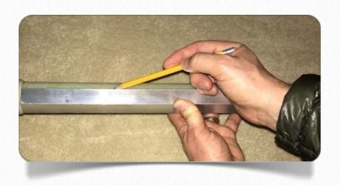
and the other about 24" forward from the aft end of the rocket. Then trace each GLR Rail Guide on the airframe.
