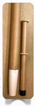
assembly and line it up correctly. The Middle Centering Ring will be Forward of the small fin slots and the Forward Centering Ring will be Forward of the large fin slots. On the outside of the airframe make a mark with a pencil where the Forward Centering Ring is and where the Middle Centering Ring is. Disassemble the GLR Pinnacle Tailcone and airframe.
