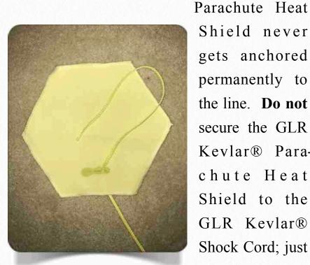
Shield never gets anchored permanently to the line. Do not secure the GLR Kevlar® Parachute Heat Shield to the GLR Kevlar® Shock Cord; just
