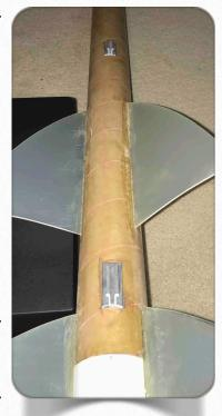
idea to place some tape on the GLR Rail Guides lightly securing them to the airframe. The tape will prevent a "drooping" of the GLR Rail Guide system as the J.B. Weld sets.
